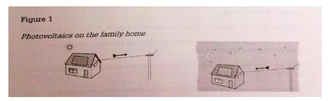
Residential use of photovoltaics – by day excess power is sent to the grid, and by night power is supplied to the home.
