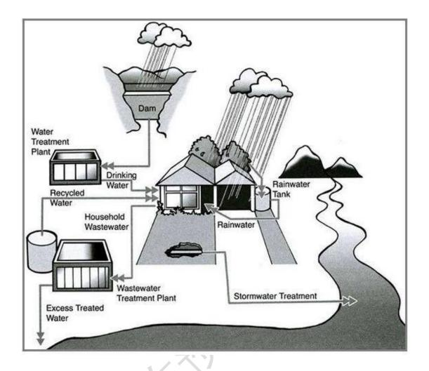
The illustration depicts different steps through which rainwater is collected, processed and released for reuse for domestic consumptions. Overall, rainwater recycling process involves various interrelated phases including the use of the dam, treatment plant, water tank and the whole process is dependent on rain pour.
