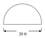
The figure above shows the dimensions of a semicircular cross section of a one-way tunnel. The single traffic lane is 12 feet wide and is equidistant from the sides of the tunnel. If vehicles must clear the top of the tunnel by at least  $\frac{1}{2}$  foot when they are inside the traffic lane, what should be the limit on the height of vehicles that are allowed to use the tunnel?
